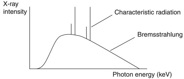
2. Characteristic radiation. This occurs when an incoming electron has sufficient energy to overcome the binding energy of one of the electrons in the metal anode atom's orbital shells. This orbital electron then "drops" into a lower energy shell, and the resulting energy loss is released as an x-ray with a particular fixed energy value.
