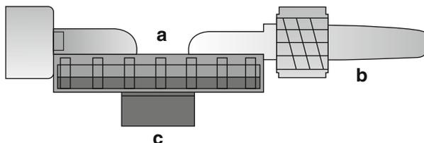
**Fig. 32.1** An example of a strain gauge external transducer system. The diaphragm lies below the housing (*a*) which goes to the patient via a water column at connector (*b*). The transducer diaphragm is placed into the housing (*c*)
