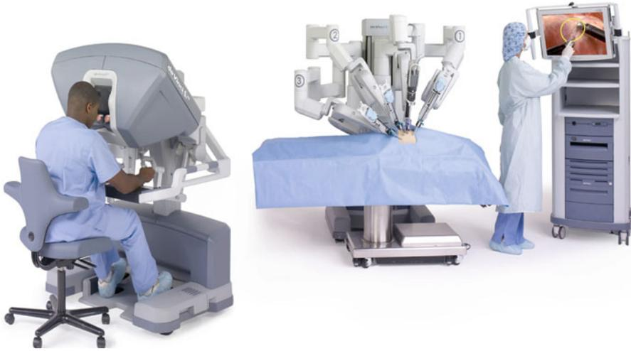
**Fig. 67.1** The three components of the da Vinci robotic operating system: the surgeon's console, the patient-side cart with four arms (*originally three*), and an endoscopic stack which also houses some of the computer hardware (Image © 2011 Intuitive Surgical, Inc.)
