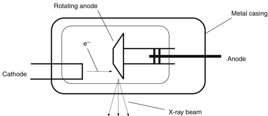
**Fig. 2.1** Schematic diagram of typical x-ray tube
