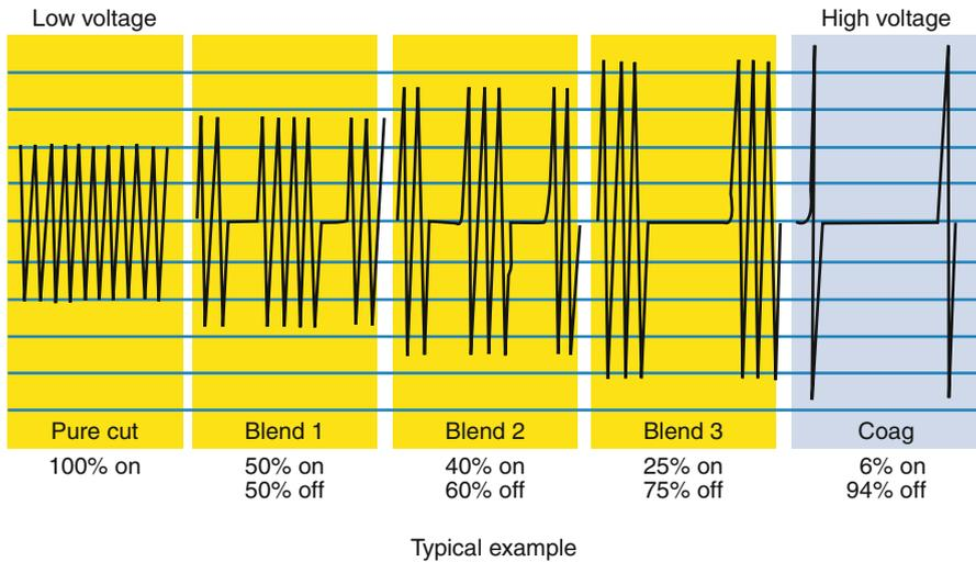
**Fig. 60.1** The relationship between voltage, waveform, and tissue effect of pure cut, blend, and coag monopolar diathermy settings
