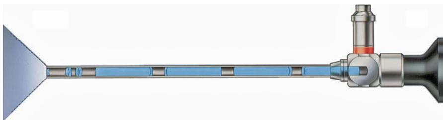
**Fig. 41.2** Hopkins rod-lens array endoscope. The lenses are shown in *blue* (Image courtesy of Karl Storz)
