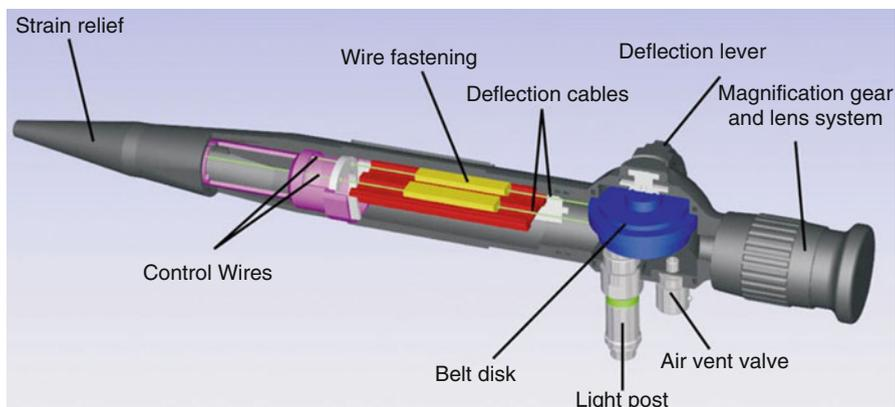
**Fig. 40.1** The control components of a flexible endoscope (Image courtesy of Karl Storz)
