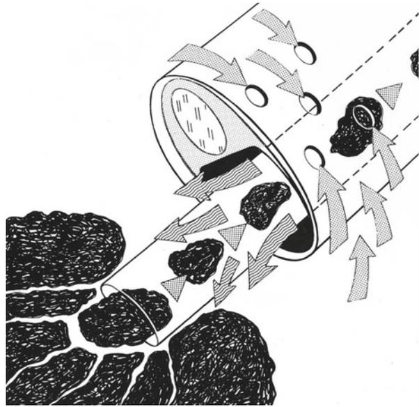
guided with precision of one micrometer, to generate ballistic energy. When the projectile hits the probe in the handpiece, a shock wave is transmitted through the probe to the calculus. The different acoustic characteristics of the metal probe and the stone lead to disintegration of hard and large stones. Electrokinetic lithotripters (EKL) use a magnetic core to create vibration at 15–30 Hz directly in the metal probe, which is placed in contact with the stone to drill it.
