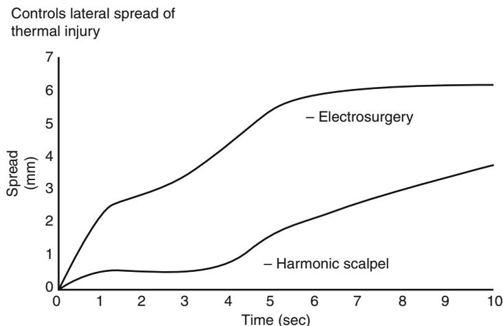
**Fig. 62.1** A comparison of the extent of lateral thermal spread for electrosurgery and ultrasonic energy used in the harmonic scalpel
