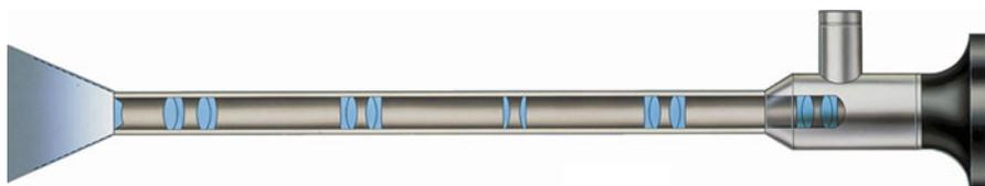
**Fig. 41.1** A simple lens endoscope as first described by Nitze. The lenses are shown in *blue* (Image courtesy of Karl Storz)
